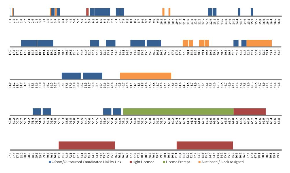
Figure 1 - Frequency bands available for use by fixed links in the UK (GHz)
