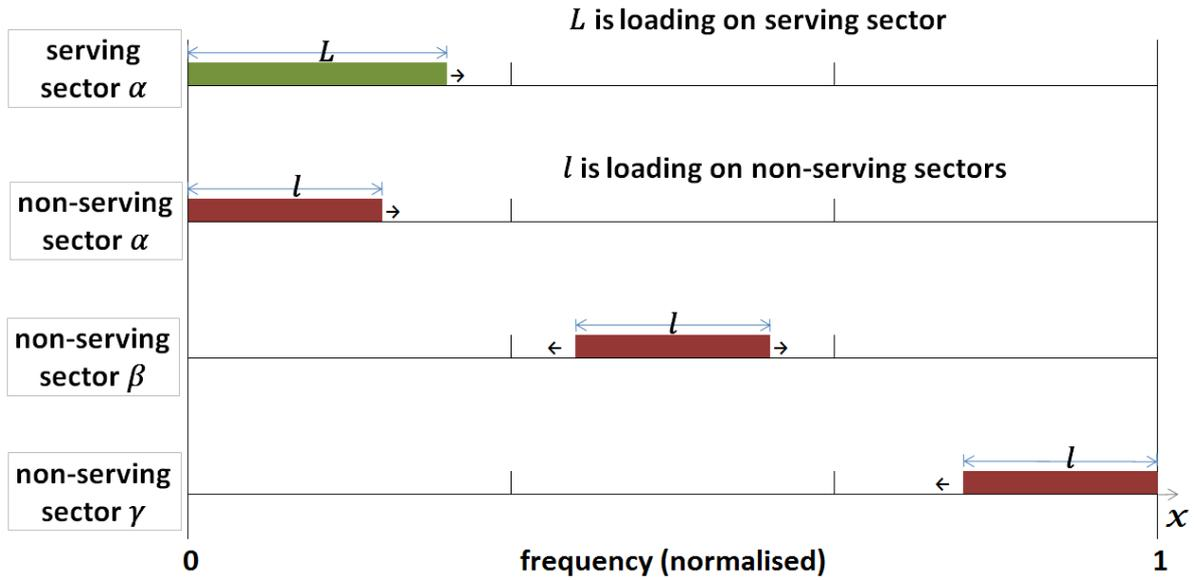
A14.77 For the purposes of this illustration (Figure 6) the bandwidth is normalised to unity, meaning that the frequency (denoted  $x$ ) lies between 0 and 1, and the sectors  $\alpha$ ,  $\beta$  and  $\gamma$  are arranged relative to frequency as shown in the diagram.
