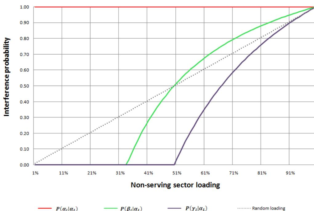
A14.81 Figure 8 below illustrates the case where the serving-sector loading is fixed at 85%. For such heavy loading we see that the interference probability does not have a great dependence on the loading algorithm chosen. However we see again that, at loadings above 50%, intelligent loading does not provide on average a lower interference probability than random loading.
