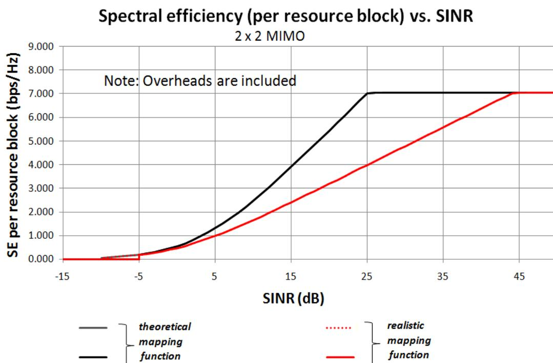
A14.110 For the generation of the (speed) single user throughput curves, the available user bit rate per resource block is calculated by multiplying the spectral efficiency by 180 kHz (the occupied bandwidth of an LTE resource block).
