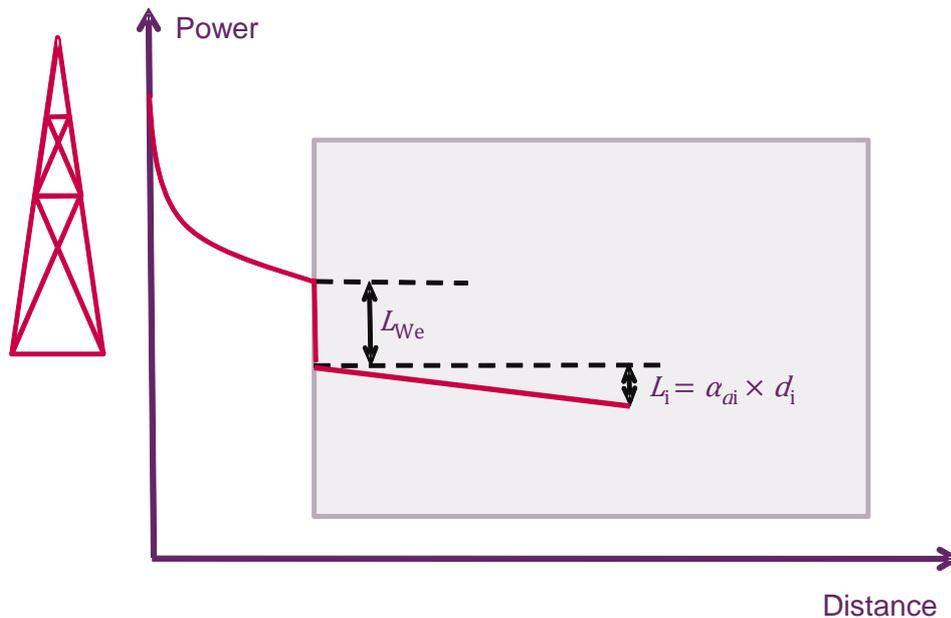
A14.39 Both the initial loss due to propagation through the external wall ( $L_{We}$ ) and the internal loss ( $L_i$ ) are uncertain and will depend in a complex way on a number of factors including:
