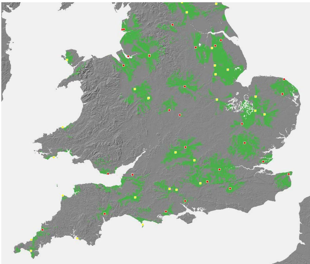
Figure 3.12: Coordination ranges for  $-45\text{dBm/MHz}$  EIRP OOB
