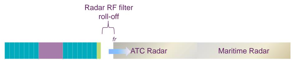
Items 1 and 2, can be mitigated by modifying the current radar fleet. Modifications are currently being developed by radar manufactures and these will include RF filters to improve radar selectivity.
