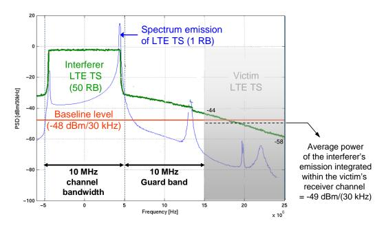
This BEM indicates that a TS in the top 10 MHz block will put an out of band emission of approx –40 dBm into a 15 kHz receiver bandwidth at 869 MHz. This would happen all across the SRD band if it were running 50 RB, or on certain channels if it were running 1 RB.
