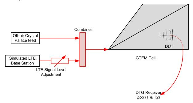
Fig.1 LTE Test Setup
