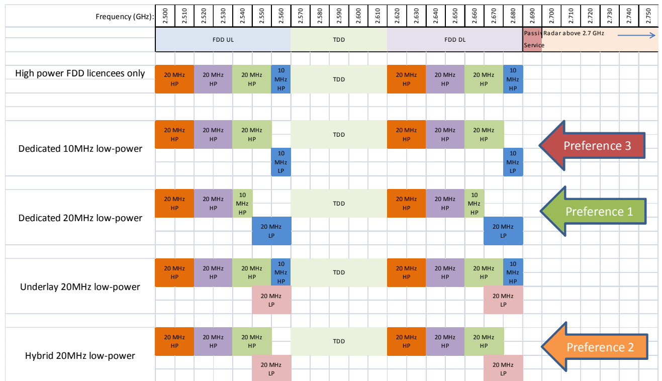
Figure 3-1: Spectrum options for the potential low power shared access channel (positioning is for illustration only)
