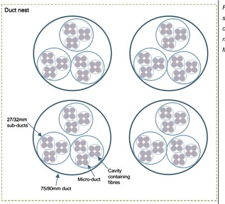
Figure 4.5: Duct nest showing potential layers of ducting within a duct nest [Source: Analysys Mason]
