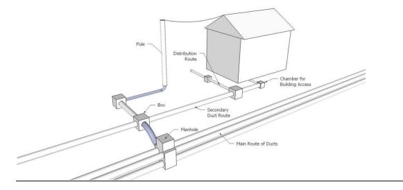
Figure 3.2: Tree and branch configuration of the access network [Source: Analysys Mason]
