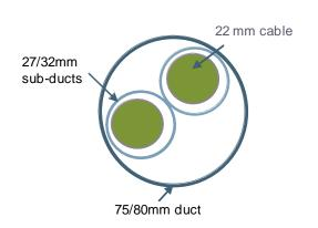
Figure 4.3: Sub-ducting of an 80mm duct for a 22mm cable [Source: Analysys Mason]
