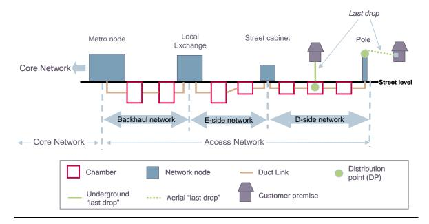
Figure 3.1: Diagrammatic representation of UK incumbent network [Source: Analysys Mason]
