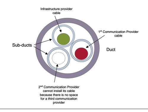
Figure 6.2: Limitations of 1:1 matching principle [Source: Analysys Mason]
