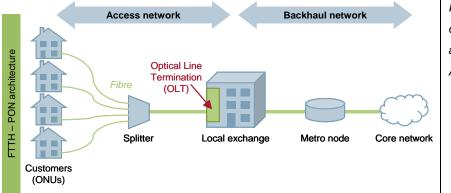
Figure 3.12: Passive optical network architecture [Source: Analysys Mason]
