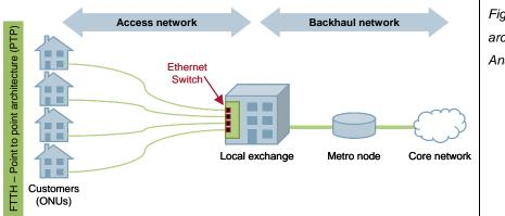
Figure 3.11: Typical PTP architecture [Source: Analysys Mason]
