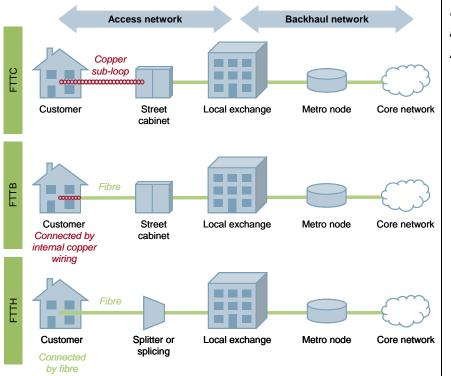
Figure 3.9: FTTx architectures [Source: Analysys Mason]
