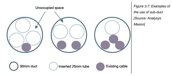
While sub-ducts reduce the absolute capacity of the main duct, it is a useful device for allowing cables to be installed and removed without risking damage to existing cables. The use of sub-ducts may become essential if more than one operator plans to share the same duct.
