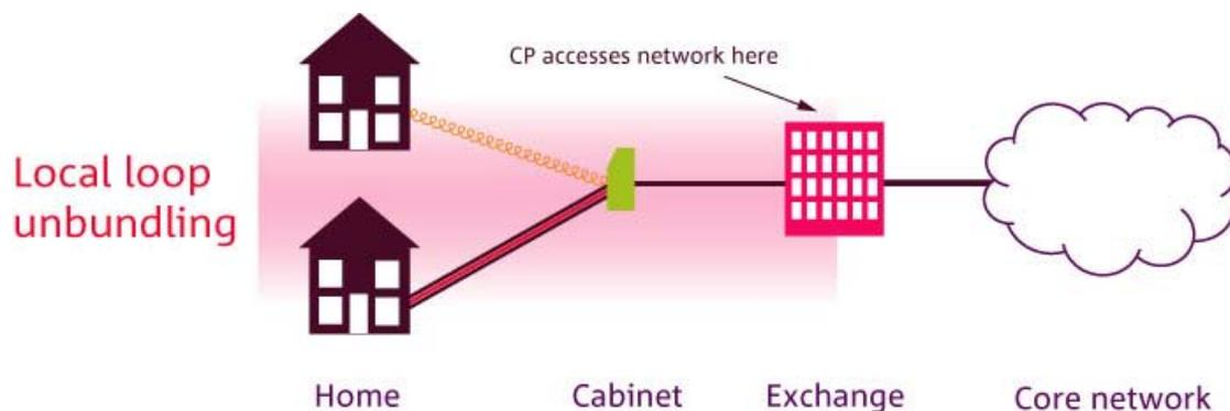
**Local Exchange / Exchange:** The local exchange refers both to a building and the equipment within it. It is the location at which local access network lines (both copper and fibre) will end, and will be connected to the relevant equipment. Exchanges may house DLEs and concentrators for voice services; DSLAMs for broadband; or MSANs for both voice and broadband in an NGN. In the BT network there are around 5,500 exchange buildings across the UK.
