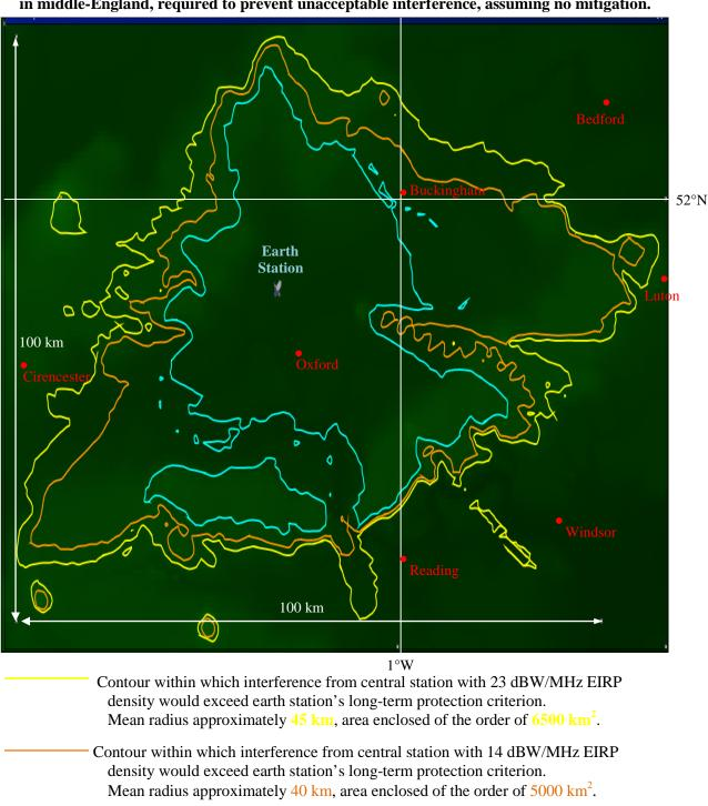
Contours showing separation distances, between Freedom4 stations and example earth station in middle-England, required to prevent unacceptable interference, assuming no mitigation.
