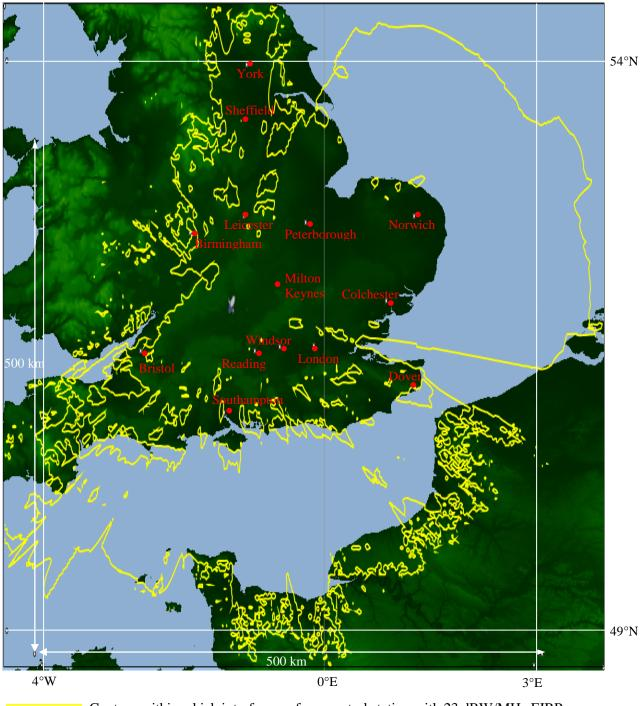
Contour within which interference from central station with 23 dBW/MHz EIRP density would exceed earth station's short-term protection criterion. Mean radius approximately 205 km, area enclosed of the order of 132000 km<sup>2</sup>.
