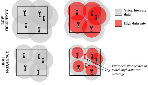
With similar cell site distribution basic services can be offered with similar coverage at both low and high frequency High speed data suffers more at higher frequency and extra cell sites are needed to match coverage of operator using lower frequency
