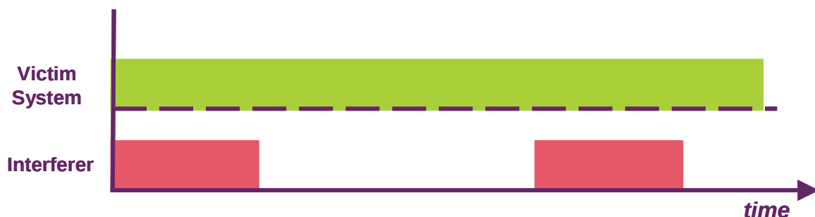
Figure 3: Interference in the time domain
