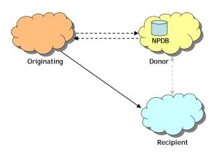
This shows a Direct Routing (DR) method without the use of a common database.
