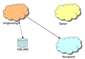
The Direct Routing case means that the donor network is not involved in routing a call to a ported number.
