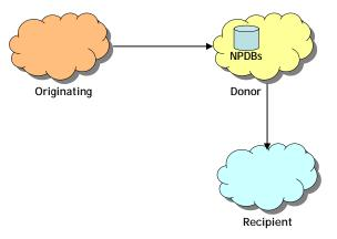
In this case, the destination number has been ported. It shows the Onward Routing (OR) method which applies to the UK fixed network today.
