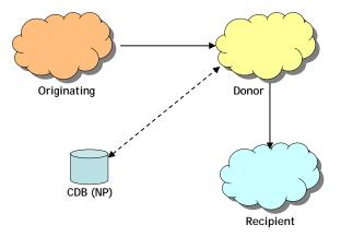
This illustrates a system where a Common Database (CDB) is used to provide the destination information. It also illustrates a case where an originating network cannot consult the CDB directly. An example of where this could occur is in a fixed to mobile call, where the mobile networks have implemented the CDB ahead of the fixed networks.
