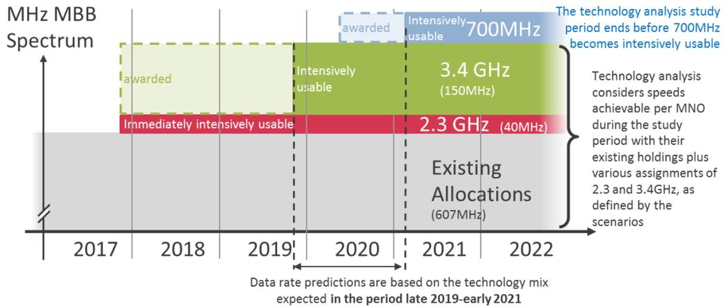
**Figure 2-1: Spectrum timing diagram in the context of this analysis**
