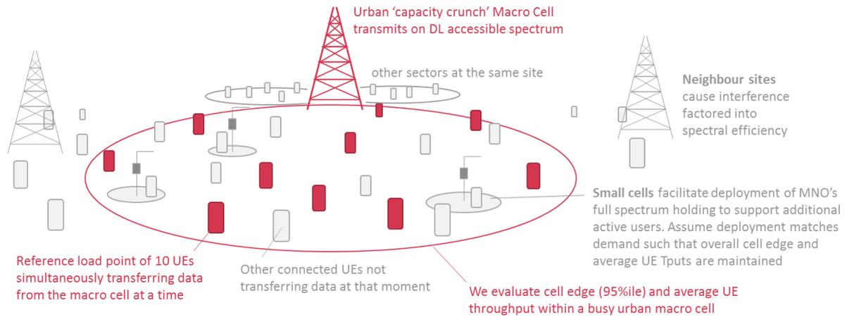
**Figure 3-1: Data rates represent cell edge and average downlink user throughputs for a busy urban macrocell**
